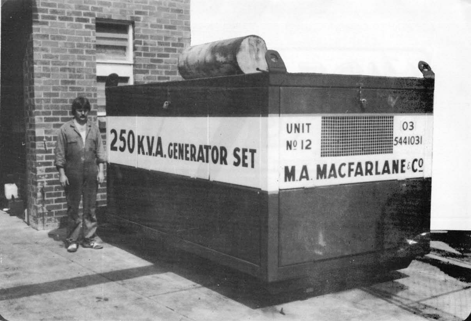
250KVA Cummins powered diesel generating Set, complete with weather proof canopy and 24 hour run fuel tanks.
